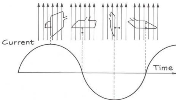
the coil continues to rotate, it includes more field lines (d) while it reaches a maximum at (e) once again. As the coil rotates, the magnetic field inside it changes, and a current is induced.
