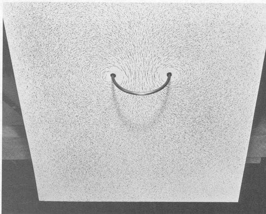
Clearly, the electric current itself gives rise to the magnetic field. Within a decade, this observation led to the development of powerful electromagnets and, ultimately, to an atomic explanation of magnetism.
