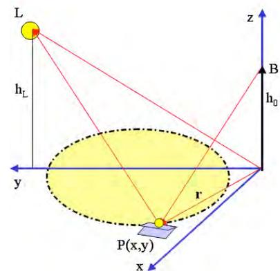
**Fig. 7: The boundary of the area lit up by reflected light depends on the heights of the light source L and the observer B and on the maximal slope of the waves**
