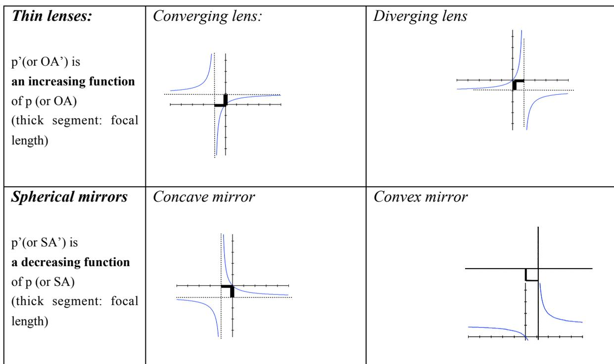
**Fig. 5. Correspondence between object and image positions for thin lenses and spherical mirrors. In each case, a hyperbola intervenes :  $FA.FA' = [-(lenses) \text{ or } +(mirrors)] f^2$ , shifted by + or - the focal length along each axis.  $OA, OA', SA, SA', p, p', FA, FA'$  are algebraic quantities.**
