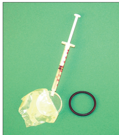
Fig. 3. Elements of the water-filled lens.
