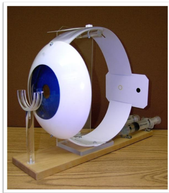
FIGURE 2. A functional model of the optical system of the human eye. Available from several sources such as http://www.universalmedicalinc.com/
