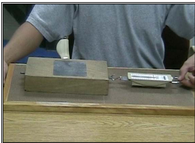
FIG. 2 (color online). Dragging of wooden block.
