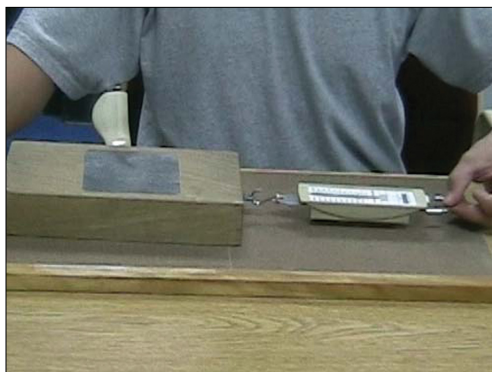
Fig. 1. Exploration Activity: A wooden block is dragged along a plank, half of which is covered with sandpaper.
