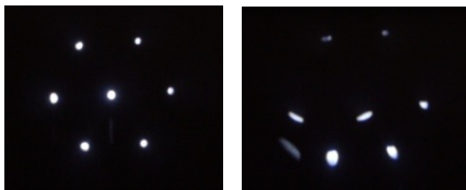
FIGURE 2. The grid on the left is a simulation of the grid from an eye with no defects, while the one on the right represents significant vision defects. (Courtesy of Prof. Hartmut Wiesner, LMU, Munich).
