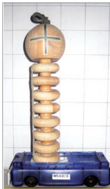
Fig. 3. The head-neck model on a dynamics cart.
