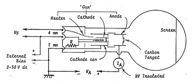
Figure 4. Schematic of the electron diffraction tube.
