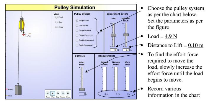
Load (N) = 4.9 N (due to the 500 g object that you are lifting)
