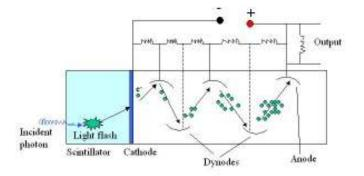
The scintillation materials in the PET detectors are chosen such that the material has practical importance when receiving the gamma ray photons of energy 511 keV. More specifically stopping power, amount of light produced against each absorbed photon and time taken for the decay of light are the important material characteristics which are considered.
