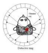
Data acquisition with a PET machine is the final step in the process. PET detectors arranged in a ring collect the signals coming out from the patient body as shown in Figure 2.1. The processing of data extracts information related to the tracer's activity in the body. Finally interpretation of results is produced in the form of scan, which is analyzed to diagnose the illness or abnormality of a tissue.
