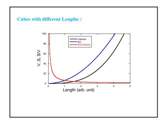
Consider a Cube with length of each side = 1m Since it has six faces, its surface area = 6 sq.m. Its volume = 1 cubic meter Surface Area to Volume Ratio = 6/1 = 6
