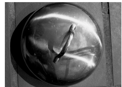
Fig. 11: Light paths on a lid deformed due to the curvature of the surface.
