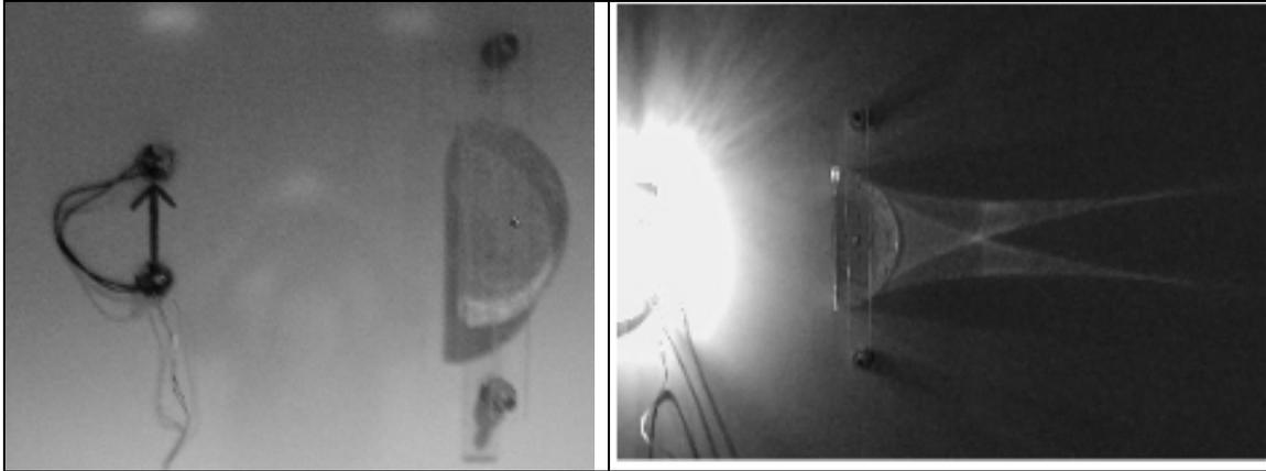
**Fig. 3 Apparatus for the Image Formation with Lenses ILD sequence, including a large acrylic, cylindrical lens and two flashlight bulbs. The right figure shows how the images of the two bulbs are formed when the bulbs are illuminated.**
