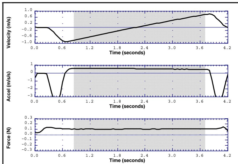
**FIGURE 1. Low friction cart moving in front of a motion detector under the influence of a force. These are actual data from an *ILD* given at Tufts. Detailed description of the experimental setup is described in the text.**
