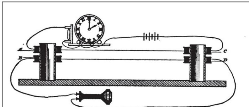
**Figure 4:** Bell’s circuit for an induction balance. For now we will focus on the coils and telephone receiver. We will investigate the purpose of the clock later. A simplified version of this circuit is shown in Figure 5. (A. Graham Bell, *Proceedings of the 31<sup>st</sup> Meeting of the American Association for the Advancement of Science*, 1882)
