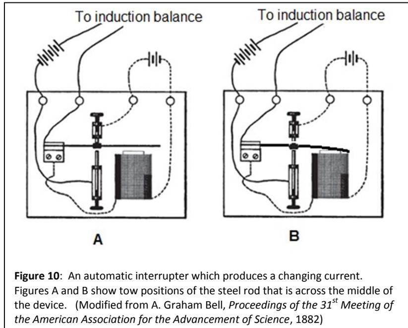
**Figure 10:** An automatic interrupter which produces a changing current. Figures A and B show two positions of the steel rod that is across the middle of the device. (Modified from A. Graham Bell, *Proceedings of the 31<sup>st</sup> Meeting of the American Association for the Advancement of Science*, 1882)
