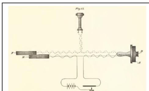
Figure 2. A drawing from one of Bell's papers showing one of the devices which he used to attempt to find the bullet in James Garfield. (From A. G. Bell, *American Journal of Science* 25 (145-150), 22-61 (1883))
