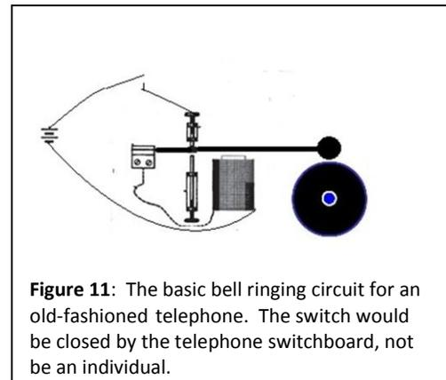
**Figure 11:** The basic bell ringing circuit for an old-fashioned telephone. The switch would be closed by the telephone switchboard, not be an individual.
