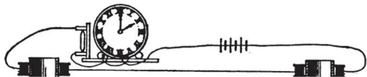
**Figure 9:** upper half of the induction balance circuit. (A. Graham Bell, *Proceedings of the 31<sup>st</sup> Meeting of the American Association for the Advancement of Science*, 1882)
