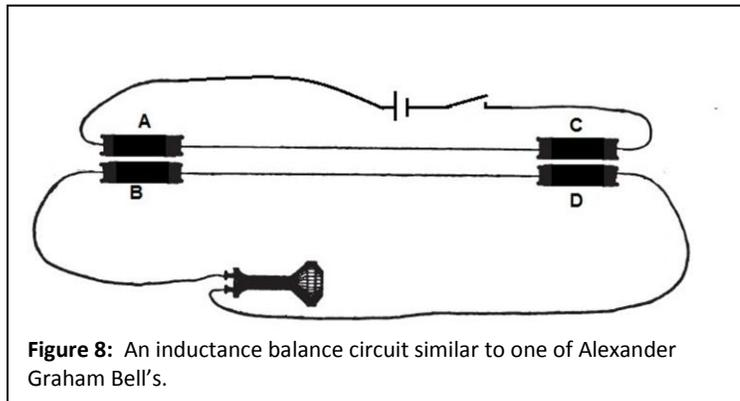
Now place a piece of metal between coils A and B. Test to see if the circuit becomes unbalanced. Then experiment with the metal to see if different locations of the metal result in different levels of a lack of balance. Record your observations below.
