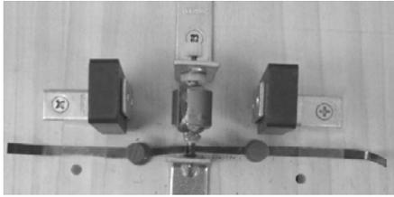
**FIGURE 1.** Permanent Magnet Board Motor (PMB)
