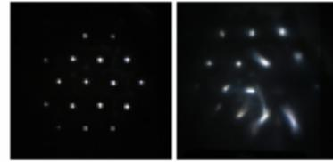
**Figure 2.** Grid pattern formed with Colicchia and Wiesner model [10] from normal lens (left) and aberrated lens (right).
