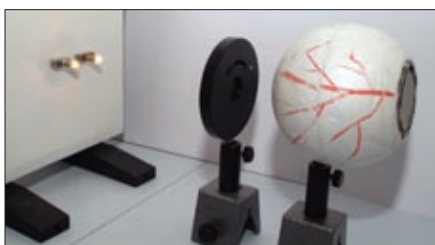
Fig. 5. Experimental device with a pinhole between the light source and the eye model.
