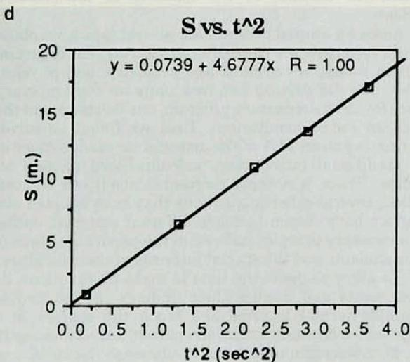
**Linearizing data** using spreadsheet and graphing software. **a:** Students drop an object from different heights  $S$ . **b:** Data are entered into a spreadsheet. **c:** Data are transferred to a graph and plotted. **d:** Vertical distance  $S$  is plotted as a function of  $t^2$ , and the curve is linearized.
