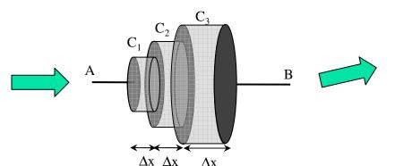
N capacitors, plates are  $\Delta x$  apart, radius of the i-th plate:  $r_i = a + bx_i$
