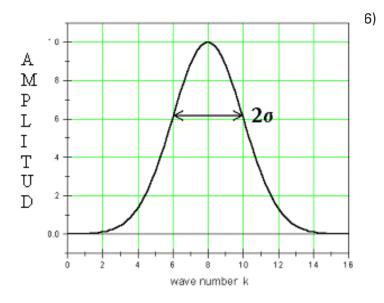
Figure 7: A Gaussian with  $\sigma=2$  and  $k_0=8$ .
