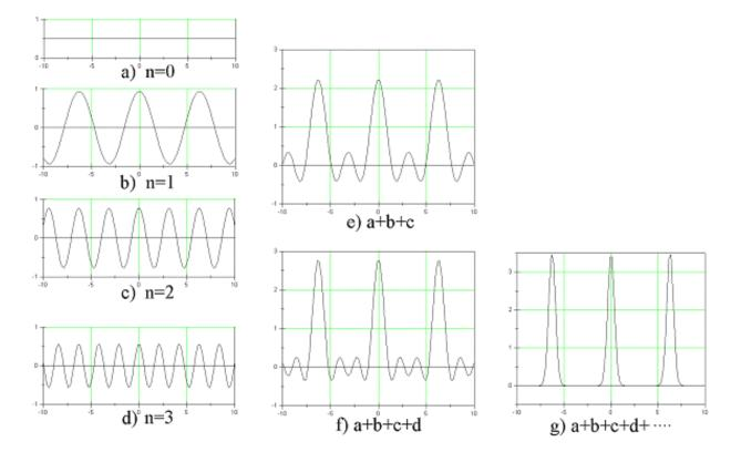
Figure 2: Adding waves a), b), and c) produces the wave shown in e). Adding in another wave, shown in figure d) results in the wave shown in figure f). Figure g) shows the wave packet resulting from the addition of ten waves, each with a different amplitude and wavelength.
