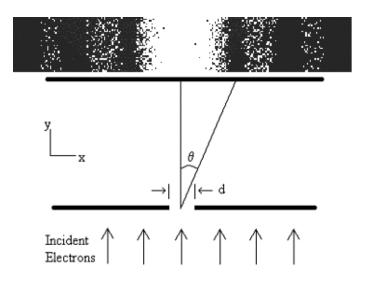
Figure 8: Electrons being diffracted as they pass through a single slit.
