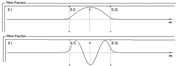
Figure 3: Some wave functions which just fit in the potential energy with minimum = -4.32 eV and width = 0.71 nm.
